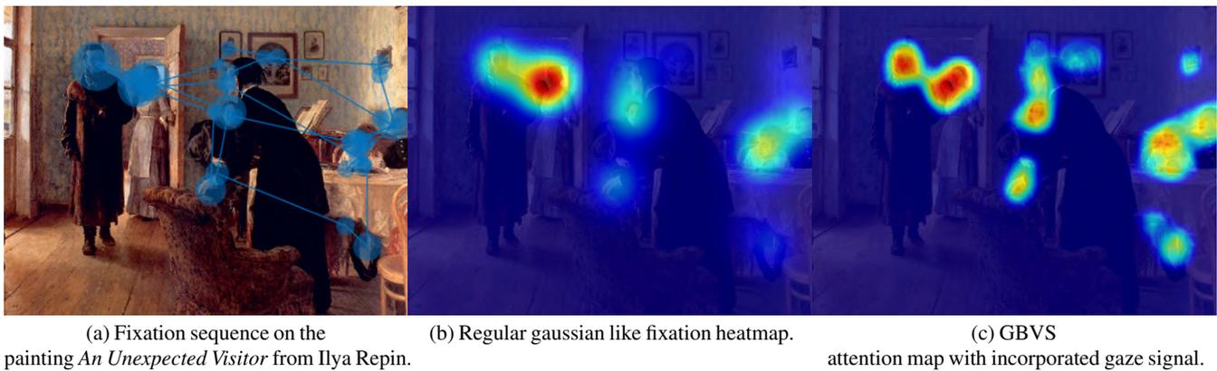
**Figure 1:** (a) shows the sequential fixation signal, where the size of the circles encodes the fixation time. (b) shows the corresponding gaussian like fixation heatmap. (c) shows the output of the proposed approach, where the tracked fixations are incorporated into the GBVS attention map calculation.
