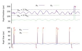
Figure 3: Rationalized outlier removal. Outliers based on subsequent pupil size (a), pupil position range (b), and pupil detection algorithm specific information (c). Notice how the pupil position estimate  $(p_x, p_y)$  is corrupted by such outliers
