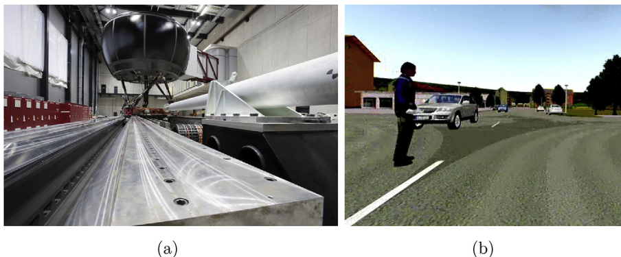
Fig. 2. Moving base driving simulator (Zeeb, 2010, pp. 157–165). (a) the entire cabin is mounted on a hexapod, moving along a 12m rail (up to 1g acceleration force). (b) Virtual reality scene as seen from inside the cabin. A pedestrian intends to cross the road from the left side (Kübler et al., 2014). Figures provided by Daimler AG.
