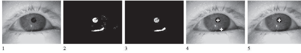
Fig. 2 Visualization of the SET algorithm. (1) input image and (2) result of binarization. (3) image after applying a region size threshold to extract pupil candidates. (4) candidate pupil centers and (5) final result.
